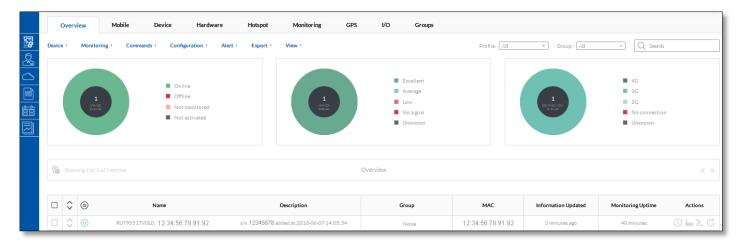
Via *Overview -> Commands ->* Access you can configure the attainment of the devices which are behind the router.
