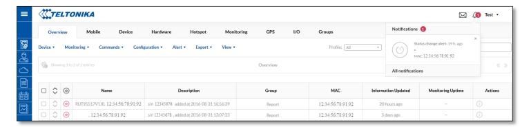
In All notifications Tab you can find previous your device events which are related to SIM switch, signal strength, device status change or mobile data usage.
