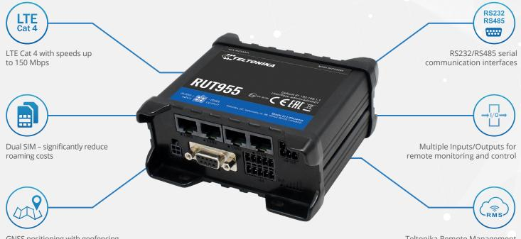
GNSS positioning with geofencing functionality
