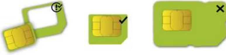
SIM card slot is designed to use with Micro SIM cards.
