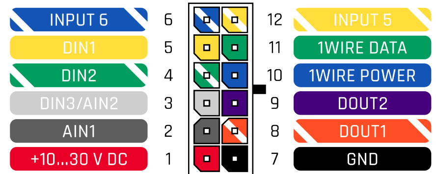
Figure 2 FMB110 2x6 socket pinout
